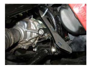
Install bracket in front of frame tubes. Fasten to plate using 10 mm carriage bolts and nuts. Do not tighten.
