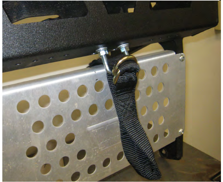
Termination strap connection to Warn front bumper.
