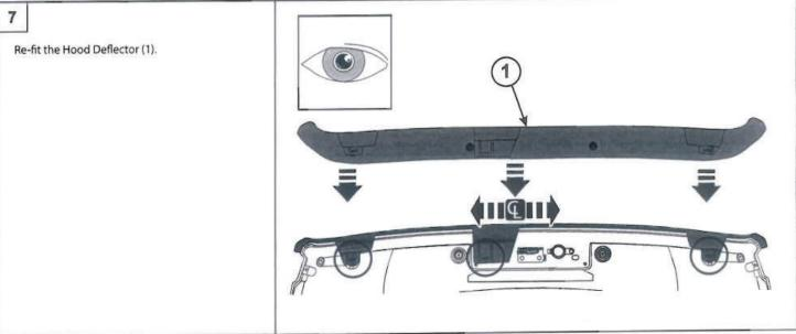
Secure the Hood Deflector with the screws and washers provided.
