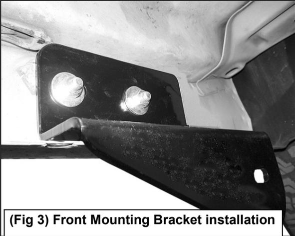
**(Fig 3) Front Mounting Bracket installation**
