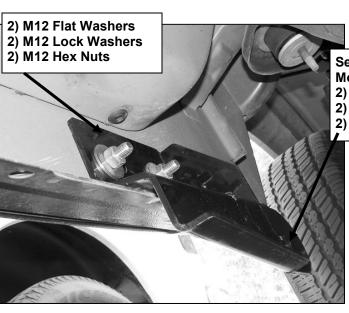
Secure the Sidebar to the Mounting Brackets with: 2) 1/2" x 2" Hex Bolts
