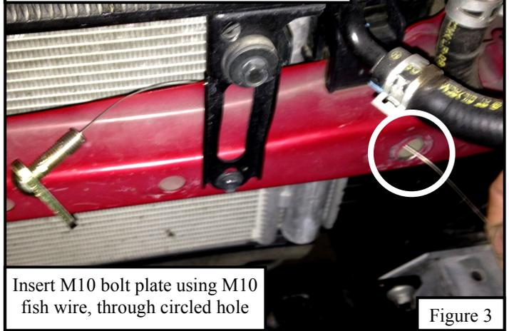
Insert M10 bolt plate using M10 fish wire, through circled hole
