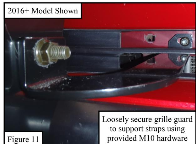
11. **For 2016+ vehicles:** Using an assistant, position the Grille Guard on the inside of Mounting Brackets and the Support Straps. Use the included (8) M10 head socket button bolts, (8) M10 flat washers and (8) M10 serrated flange nuts. Assemble loosely. See **Figures 8** and **Figure 9**. Refer to **Sportsman Grille Guard Assembly**.
