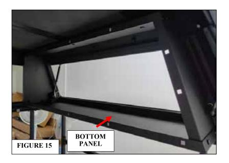
12. Adjust the Bottom Brackets location to line up the slot holes on the Bottom Panel. Attached the Bottom Panel to the Brackets with (6) M8 x 25mm Combination Bolts, (6) M8 x 20 x 2mm Flat Washers, (6) M8 Hex Nut, (Fig 16 & 17). Do not tighten hardware.
