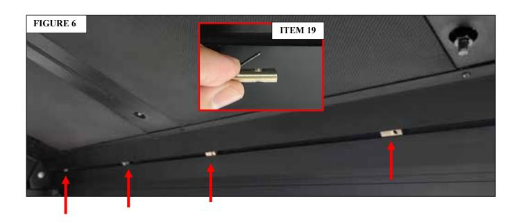
6. Attach (1) M6 Button Head Bolt, (1) M6 Lock Washer, and (1) M6 x 22 x 2mm Flat Washer to each Slot Nut, (Fig 7). Adjust the M6 bolt and nut to the appropriate position. The distance between two bolts is 300mm.
