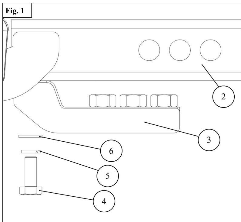
3. Slide the bracket assembly into the receiver hitch of your vehicle. Secure bracket using the receiver pin (not included).
