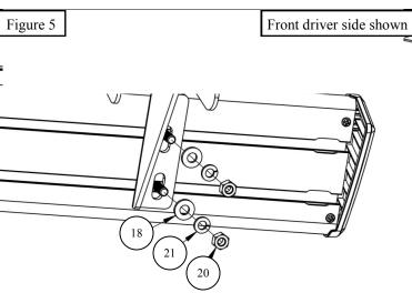
9. Align step bar and brackets to desired positioning then torque and tighten all M8 hardware to 16 ft-lbs.
