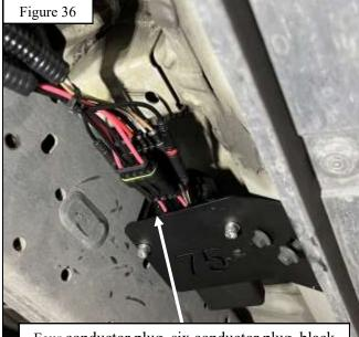
Four conductor plug, six conductor plug, black two conductor plug, and red two conductor plug connected to the control module
