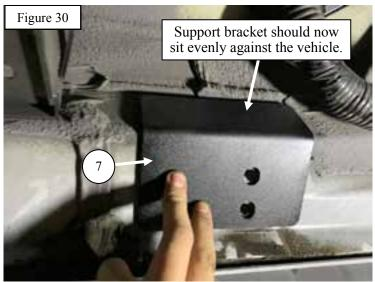
17. Install the Rear Reinforcement Bracket Plate (Item 7) to provide extra support to the rear bracket. To achieve a flush reinforcement bracket install cut away any bumps of rubber on the vehicle that prevent an even mounting position with a Stanley knife. (Figures 29 & 30)
