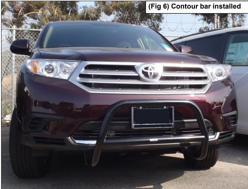
(Fig 6) Contour bar installed
