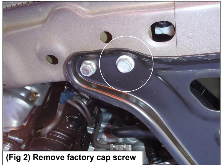
**(Fig 2) Remove factory cap screw**
