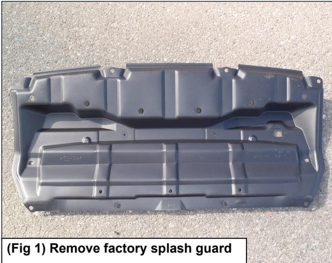
**(Fig 1) Remove factory splash guard**
