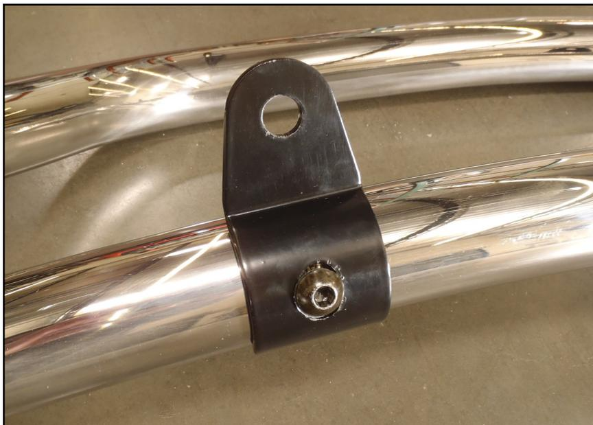
**(Fig 8) Light tab installed on bar**
