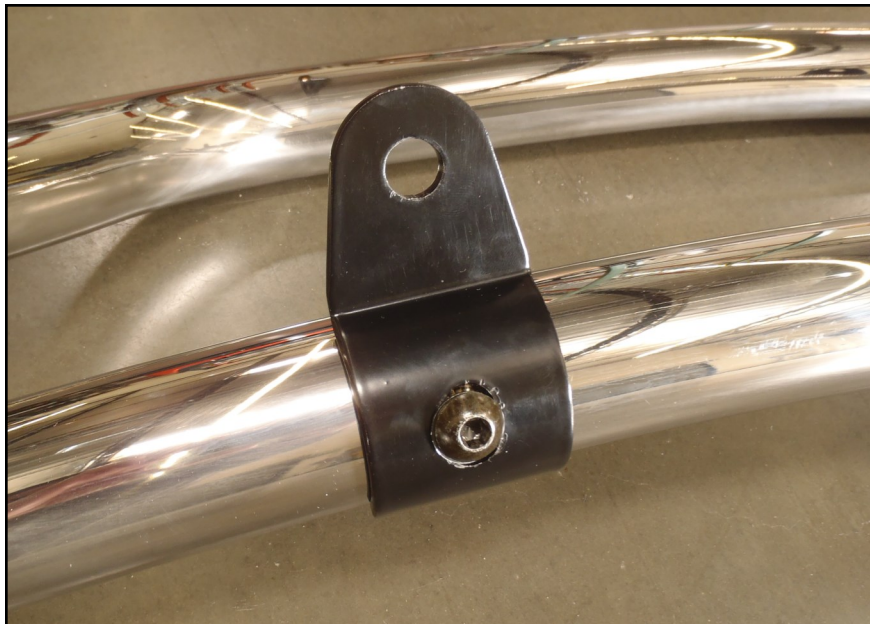
(Fig 8) Light tab installed on bar
