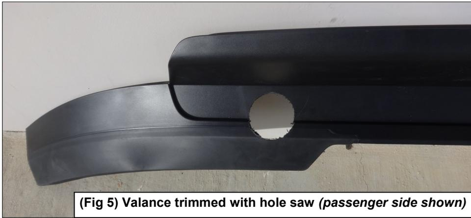
(Fig 5) Valance trimmed with hole saw (passenger side shown)
