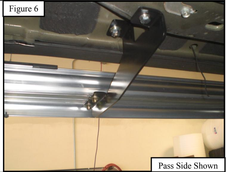
8. Once all brackets are mounted, insert supplied square head bolts into running board rails. Align bolts with slots in the mounting brackets and place board on mounting brackets. See **Figure 7 & 8**.
