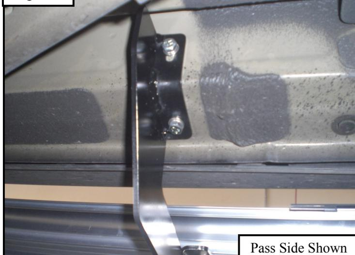
4. Look for M8 threaded holes on the rocker panel towards the center of the vehicle, as well as on the frame towards the center of the vehicle (passenger side). See **Figure 3 & 4**.
