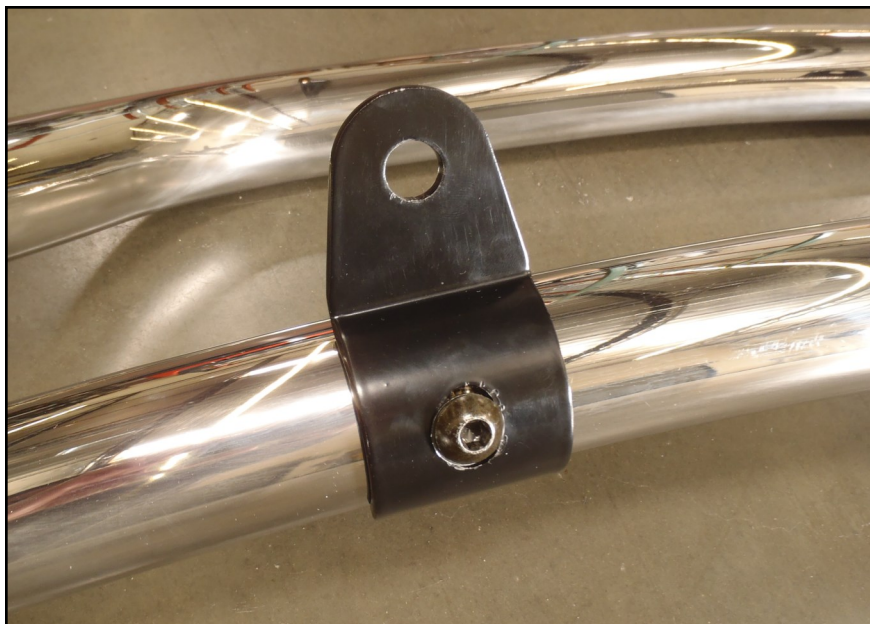
(Fig 8) Light tab installed on bar
