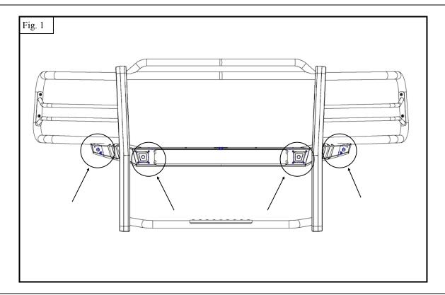
3. Starting on the passenger side, install the farthest right side sensor on to the right wing. Use the passenger wing bracket (6) and supplied M5 hardware. *Note:* Be sure to cut a piece of the supplied tape and insert between the bracket and sensor. See Figure 2. DO NOT OVER TORQUE AS IT MAY CAUSE DAMAGE TO THE SENSOR.
