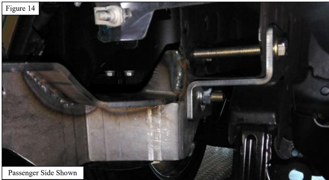
14. With help, loosely assemble the grille guard using supplied M10 and M12 hardware. **See Figure 15.**
