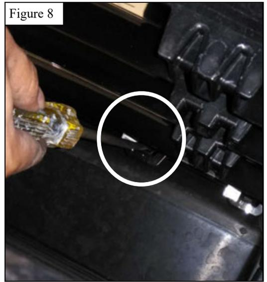
8. Remove the upper core support cover under the hood using a trim removal tool. There are multiple retainers that hold this piece on. See Figure 9.
