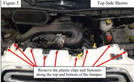
7. Remove the license plate and factory license plate holder. Remove the two bolts and carefully pull off the bumper assembly. See **Figure 6 & 7** for reference. <u>Note:</u> Make sure any wiring connectors secured to the bumper are unplugged prior to removal.
