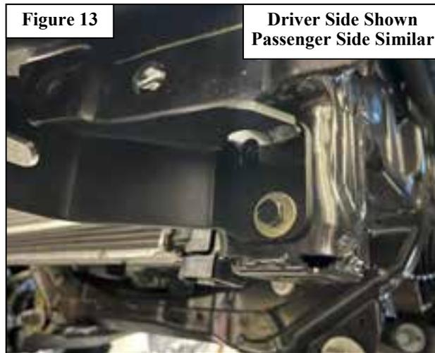
11. Using the assistance of a floor jack, lift the front bumper into position. Loosely assemble the provided M12 hardware, securing the bumper to the main brackets. Be sure not to torque the bolts allowing for alignment in a later step.
