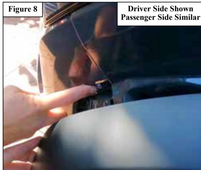
6. Remove the (8) 10mm bolts located on the bottom side of the front grille. There are (3) bolts on either corner of the bottom bumper, and (2) bolts located in the center, on the back edge of the plastic skid plate. Carefully pry the front grille off the upper clips and remove the grille.
