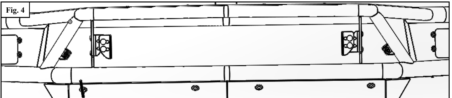
Figure 4 is an example showing the LED brackets adjusted in for the shortest light bar configuration.
