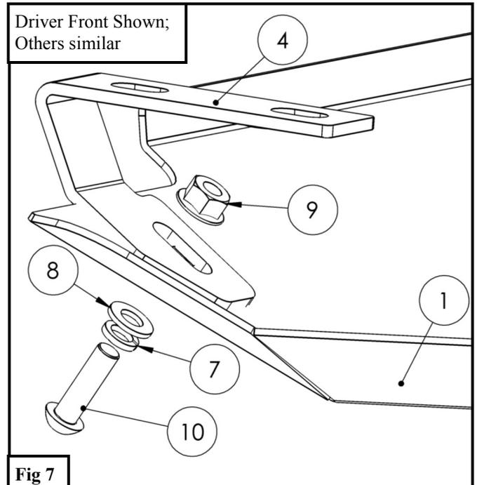
11. Align the Skid Plate as desired, then torque all hardware as specified: M10 to 38 ft-lbs, M12 to 60 ft-lbs.
