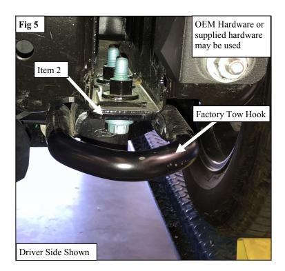
6. Align and tighten all hardware as specified: M10 to 38 ft-lbs, M12 to 65 ft-lbs
