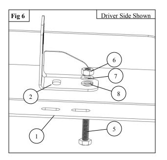
5. Align and tighten all hardware as specified: M8 to 18 ft-lbs, M10 to 38 ft-lbs.
