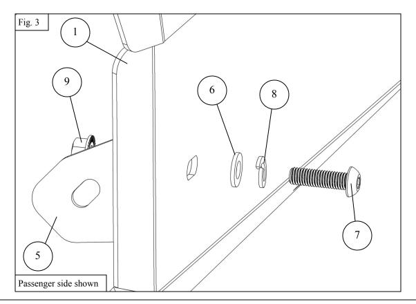
Adjust as needed and torque all M10 Hardware to 38 ft. lbs
