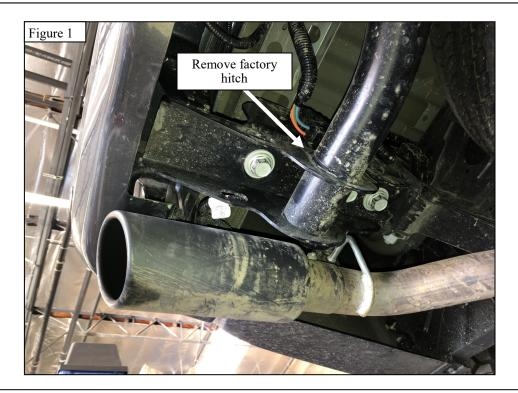
4. Using factory hardware, mount the hitch to the frame. Note: Ensure that the outlaw bumper brackets are mounted in between the frame and hitch. See Figure 2-3.
