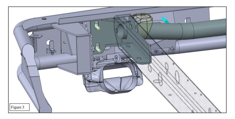
4. Adjust the bumper and hitch assembly ass necessary. Torque all hardware as specified: M12 to 55-60 ft-lbs., M14 to 90-100 ft.—lbs.
