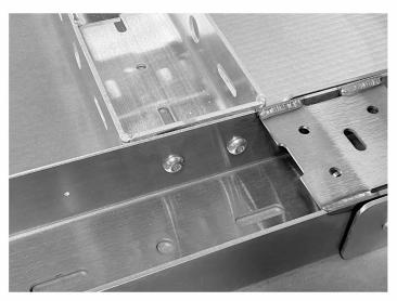
3. Connect one side of both of the longitudinal cross bar as shown. Use (2) 3/8"x1" button head bolts and flange lock nuts. Torque to 30 ft/lb.
